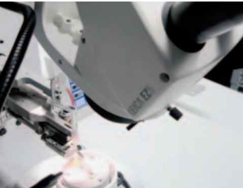
Leica EZ5 mounted to a bonder machine
